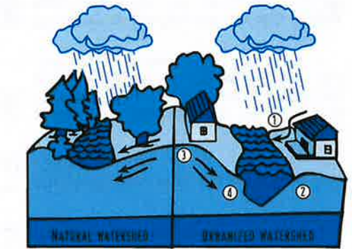
① INCREASED RUNOFF ② STREAMBANK EROSION ③ DECREASED INFILTRATION ④ DECREASED GROUND WATER FLOW TO STREAM
